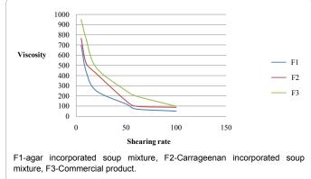
Figure 1: Viscosity of three different soup mixtures at different shearing rates.
