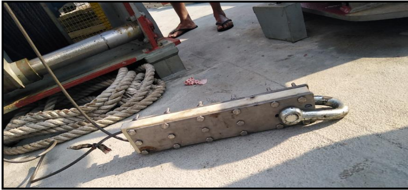
Figure 02: Fabricated load bearing connector (Guy grip dead end), between CTD and winch
