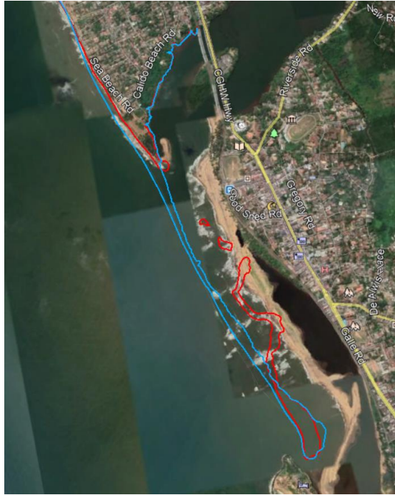
Figure4. 14: Sand barrier collapse (Blue - January 2017 & red - December 2017)
