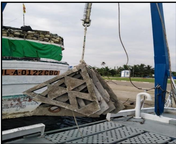
Figure 03: testing of load bearing capacity using weight know concrete slices
