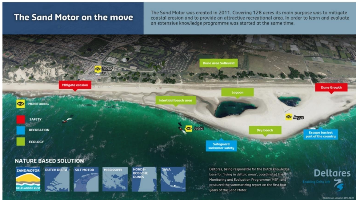
Figure 2: An example of mega sand nourishment in progress in the South Holland in the Netherlands
