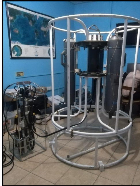
Figure 06: Testing of automated Nisking bottle operating mechanism
