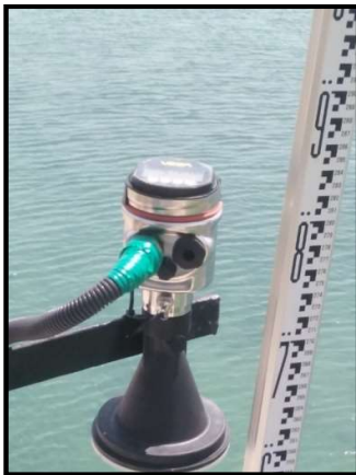
Figure 07: Acquisition of water level using radar sensor installed at Point Pedro fisheriesharbor.
